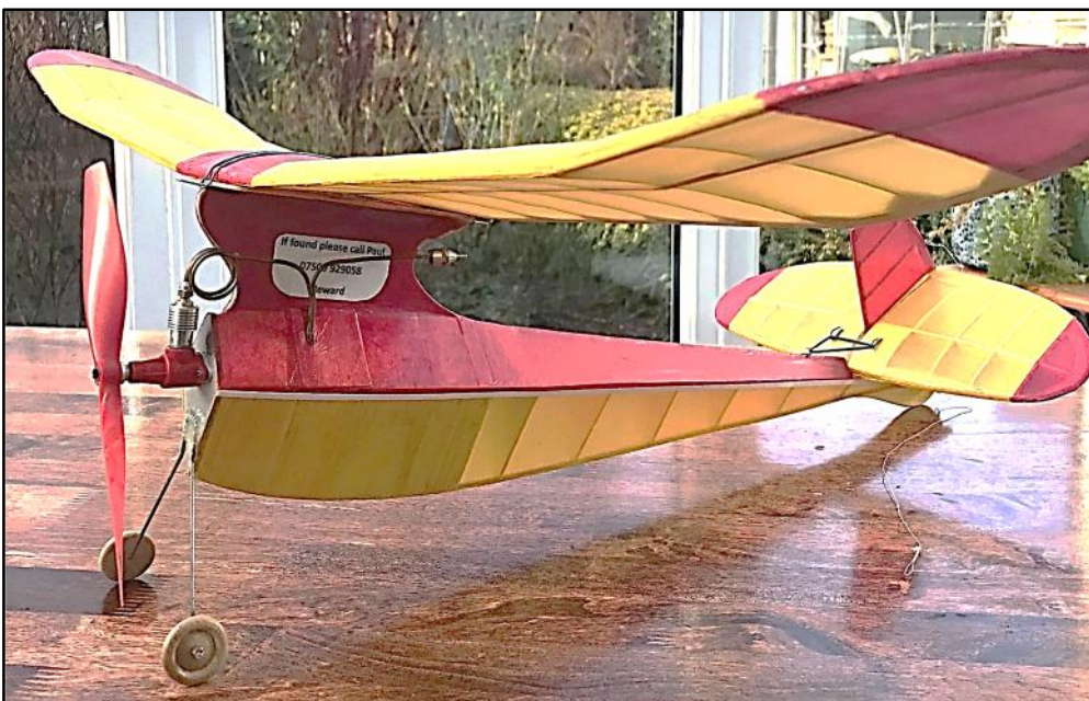
Aerbo almost ready for action. Simple motor installation allows easy adjustment of down and side thrust.
